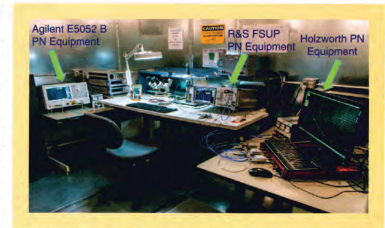
Figure 13. Ultra-low phase noise setup in Faraday cage: phase noise measurement of 100-MHz OCXO using Agilent E5052B, Rohde & Schwarz FSUP 26, and Holzworth for understanding the speed and dynamic ranges of the equipment.
